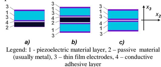
Legend: 1 - piezoelectric material layer, 2 - passive material (usually metal), 3 - thin film electrodes, 4 - conductive adhesive layer
