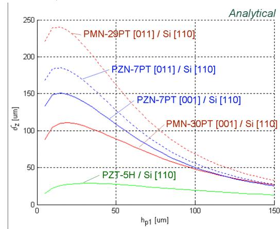
**Figure 3.** Analytical comparative diagram of  $\delta_z$  free tip displacement. Piezoelectric layer is 0.1 mm thick, length is 5 mm, width is 0.3 mm and applied voltage 80V. Silicon layer thickness  $h_{p1}$  is varied from 5 to 150  $\mu\text{m}$ .
