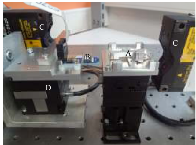
Fig. 8: Experimental apparatus including (A) compliant platform, (B) force sensor, (C) laser position sensors, and (D) NanoCube XY stage
