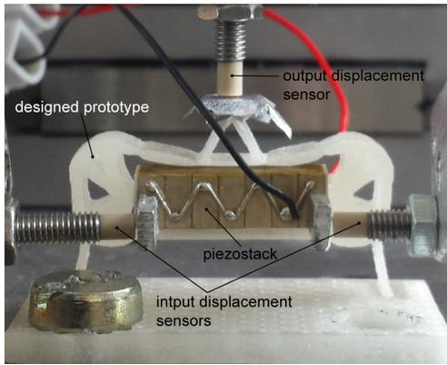
Fig. 8. Experimental bench picture.
