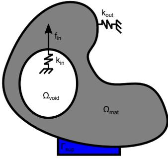
Fig. 1. Mechanical modeling of a topology optimization problem.
