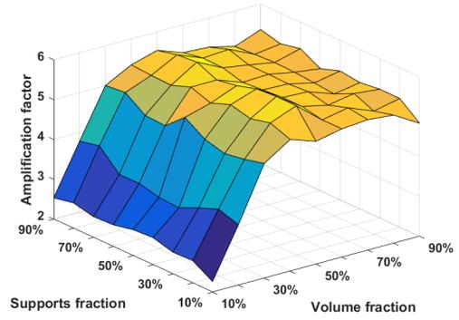
Fig. 5. Estimated amplification factor of designs. Volume and supports fraction ranged from 10% to 90%.
