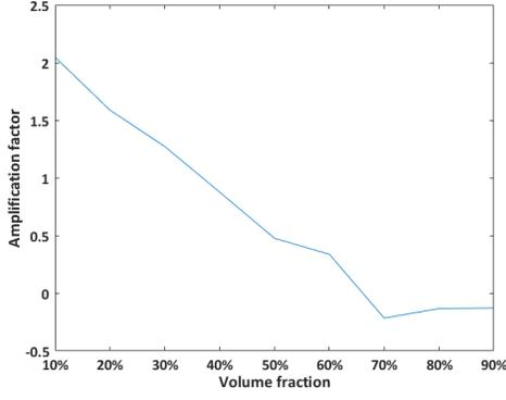
Fig. 6. Estimated amplification factor of designs. Volume ranged from 10% to 90% with 50% supports.
