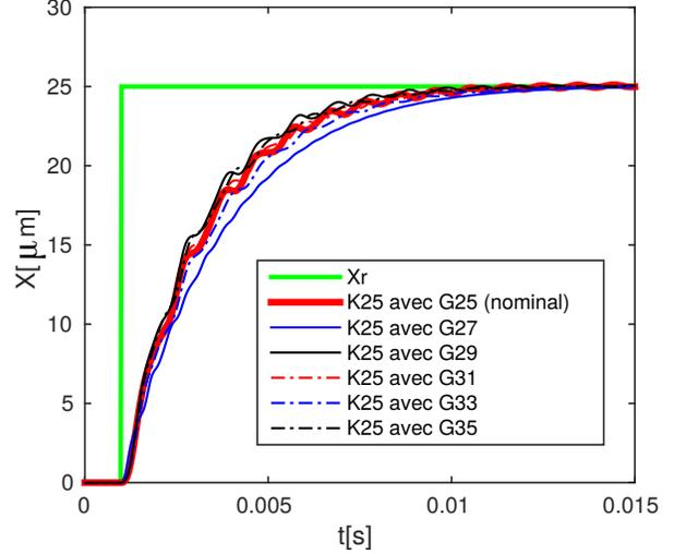
Fig. 8: Simulations of the step responses when only the nominal controller  $K_{25}(s)$  is used.
