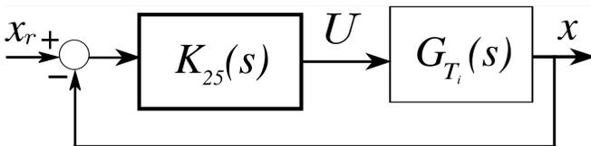
Fig. 7: The implementation scheme of the Proportional-Integral controller with the actuator subjected to the variation of the temperature.
