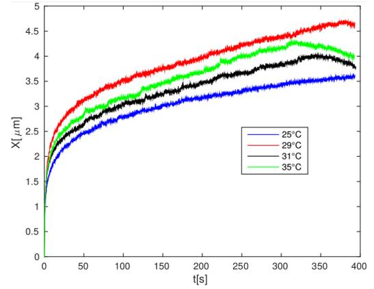
Fig. 5: The experimental characterization of the creep at different temperatures.
