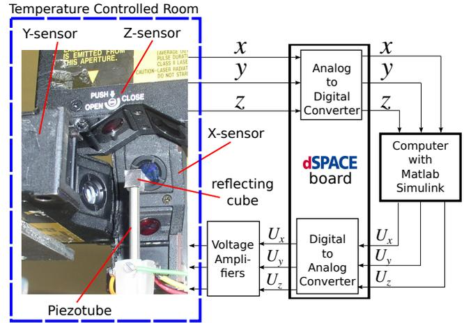
Fig. 2: The description of the experimental setup.
