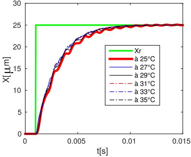
Fig. 10: The simulated step responses for the system controlled by the Proportional-Integral controllers combined with the switching strategy.
