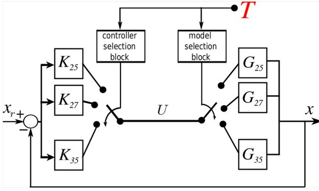
Fig. 9: The simulation scheme of the combination of the Proportional-Integral with the switching strategy.
