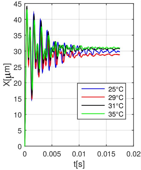
Fig. 3: The experimental characterization of the step responses for X-axis at different temperatures.
