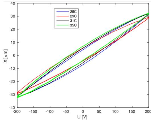
Fig. 4: The experimental characterization of hysteresis at different temperatures.
