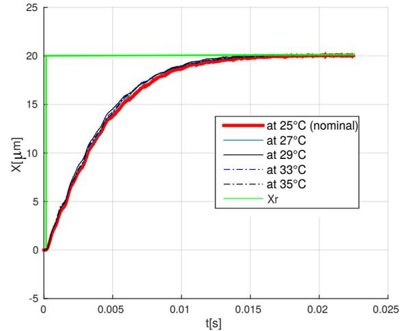
Fig. 12: Experimental step responses when the Proportional-Integral is combined with the switching strategy.
