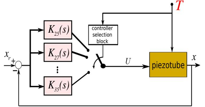
Fig. 11: The experimental implementation scheme of the Proportional-Integral combined with the switching strategy.
