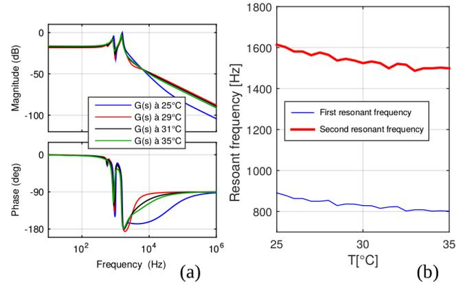
Fig. 6: The characterization of the effect of the temperature on the actuator dynamics.
