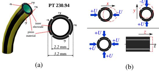
Fig. 1: Description and working principle of the piezoelectric tube. (a) Perspective and top views of the tube, (b) Working principle: application of voltages  $U$  and  $-U$  in order to get deflections along X, Y and Z axis.
