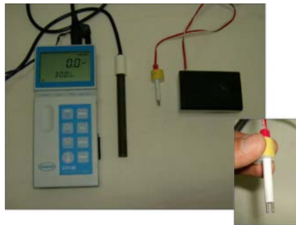
Figure 3: Photographs of the reference CO150 conductivity meter and of the designed device. Close-up of the sensing probe.
