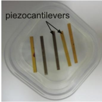
Fig 1: Photography of unimorph piezocantilevers.
