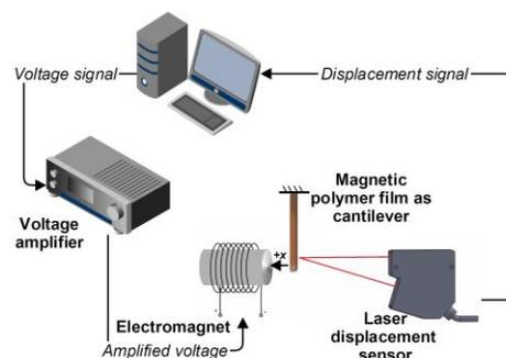
**Figure 2.-** Schematic diagram of the setup to perform the displacement measurements of the PVB/ $\text{Fe}_2\text{O}_3$  films
