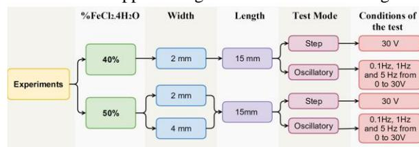
**Figure 3.-** Experimental design for the dynamic characterization
