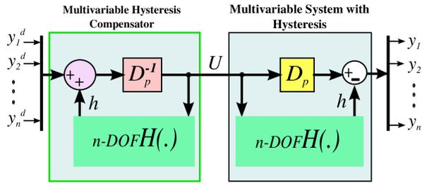
Fig. 2: n-DOF hysteresis compensator diagram.
