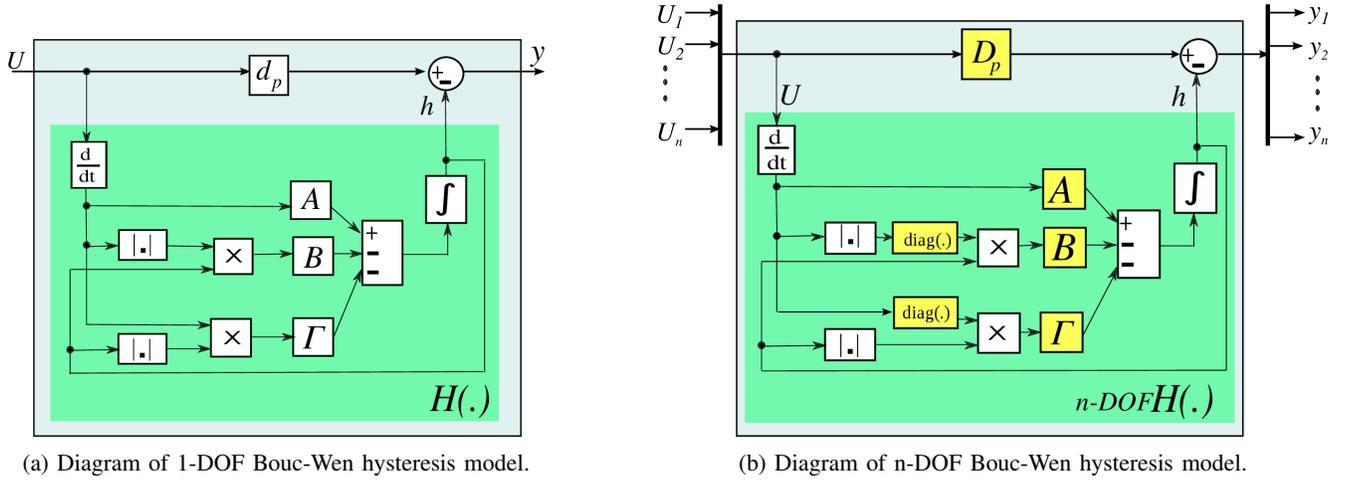
Fig. 1: 1-DOF and n-DOF Bouc-Wen model implementation.
