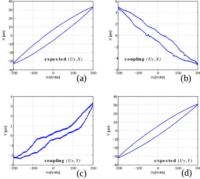
Fig. 5: Hysteresis Characterization: (a) and (c) represent  $X$  and  $Y$  displacements when only  $U_x$  is applied ( $U_y = 0$ ), and (b) and (d) when only  $U_y$  is applied ( $U_x = 0$ ). (a) and (d) represent the direct hysteresis, and (b) and (d) represent the couplings.
