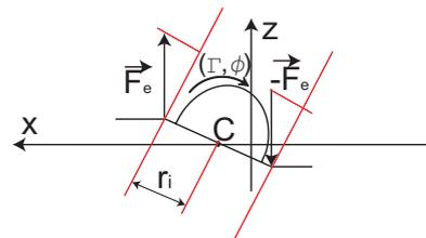
Fig. 6. Representation of the equivalent radius  $r_a$ .
