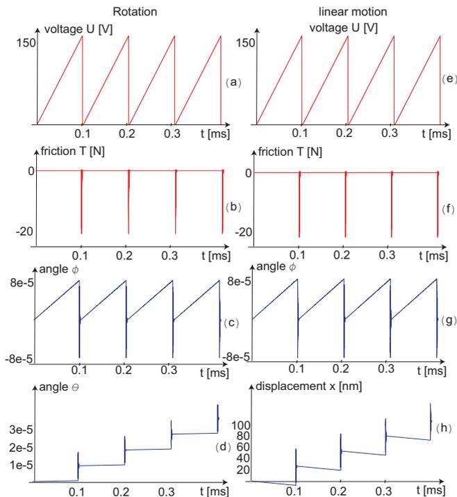
Fig. 14. Different results of simulation. a and e : applied voltage with frequency equal 9800Hz. b and f : evolution of the friction in angular and linear motion, during *stick*, its value is very low. c and g : evolution of the hemisphere rotation. e and h : evolution of the microsystem respectively in angular and linear motion.
