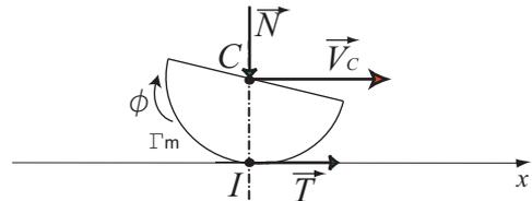
Fig. 11. The hemisphere in linear motion mode.
