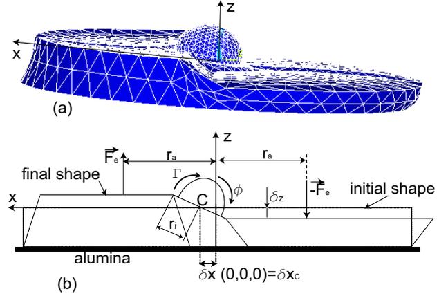
Fig. 5. Functioning of the microactuator. a : result of simulation using Finite-Element-Method. b : simplified scheme in  $Oxz$  plan.
