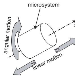
Fig. 1. Kinematical scheme of a microstation :a microsystem can rotate around Oz axis and move along it.
