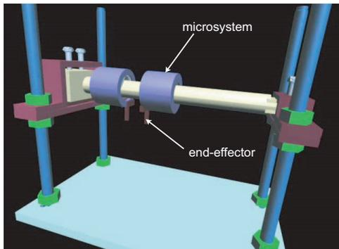
Fig. 15. When several microsystems are used, complex tasks may be done. Here, two microsystems are used in order to process *pick-and-place* task. The figure represents the principle of the future microstation studied in *Flexible Microfactory Project*.
