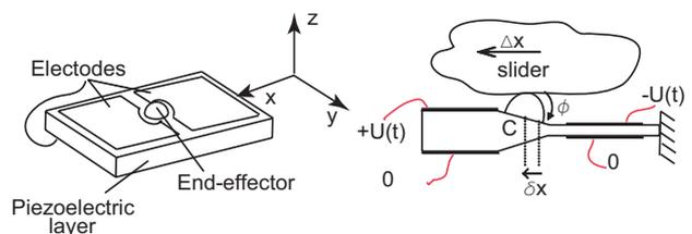
Fig. 2. Principle of the microactuator.
