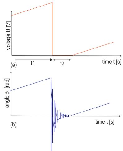
Fig. 13. a : introducing of a delay  $t_2$  in *skid* phase. b : the *slip* phase restarts when vibrations are nearly damped.
