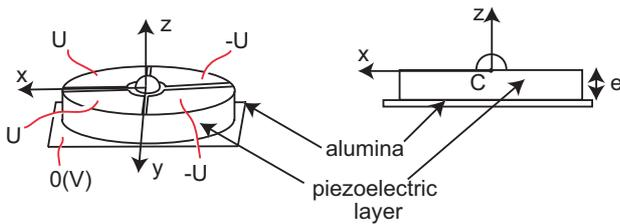
Fig. 3. Configuration of the electrodes for 2DoF.
