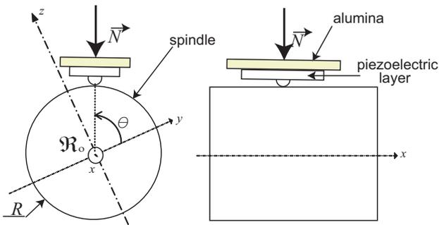
Fig. 9. Simplified scheme to study the motions of the microsystem.
