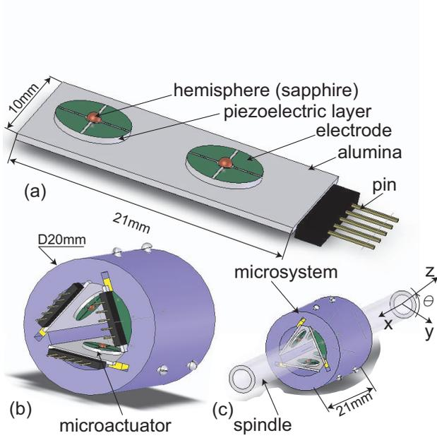
Fig. 8. a : two actuated end-effectors on an alumina plate. b : three plate of alumina spread out 360° for the microsystem. c : the microsystem has two DoF.
