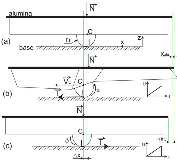
Fig. 7. a : the microactuator placed on a base. b : rolling without sliding of the end-effector (hemisphere). c : skid of the end-effector.
