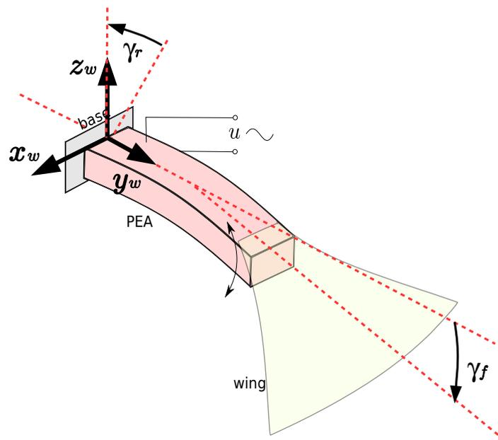
**Figure 10.** Perspective Piezowing: the PEA actuates directly to flap microrobot's wing. The flapping angle and wing's lift attitude respectively stand for  $\gamma_f$  and  $\gamma_r$ . The latter angle is generated by a PEA-based joint located at Piezowing's base.
