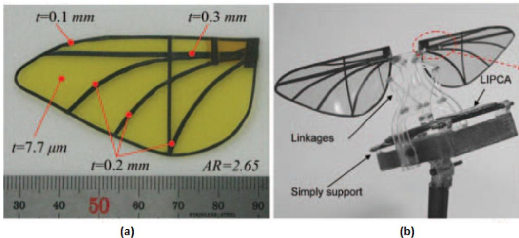
**Figure 9.** (a) Artificial Hawkmoth wing; (b) Fully assembled flapping system [64].
