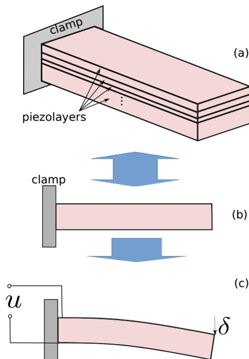
**Figure 1.** A piezoelectric cantilevered actuator. (a) Isometric scheme depicting the PEA’s piezolayers; (b) Side view of a PEA; (c) bending displacement resulting as a result of the application of an input voltage  $u$ .
