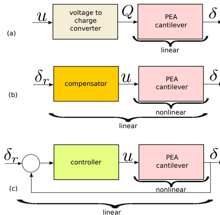
**Figure 3.** Displacement control of a PEA actuator. (a) Charge control considering that relationship of the PEA's charge and displacement are linear; (b) Feedforward control structure via a hysteresis/creep compensator; (c) Feedback control structure based on the displacement error.
