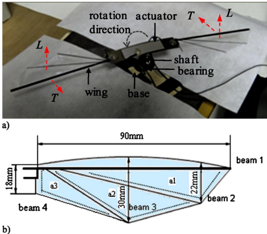
Figure 8. (a) The proposed configuration; (b) Geometric dimensions of the flapping wing [60].
